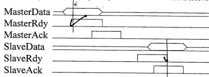
(a) To test your understanding of the signaling conventions, indicate on the above timing diagram the earliest time it is safe for the subsystem to latch MasterData and the earliest time it is safe for the subsystem to step asserting slaveData (2 points).
