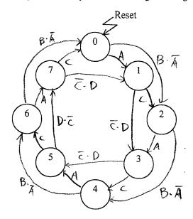
(b) Implement this state machine as a pure jump counter, showing how you wire the multiplexers and the contents of the jump ROM (4 points):
