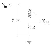
(b) With R=1 K $\Omega, L=100$  mH, C=3  $\mu$ F, sketch the frequency response of the voltage magnitude gain from  $\mathbb{V}_{in}$  to  $\mathbb{V}_{out}$ . Use the log-log scale graph-paper supplied below.
