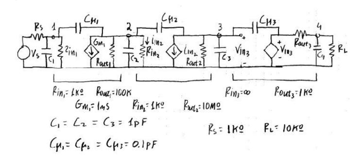
a) Find the low frequency voltage gain vout/vin. (this means that you can ignore all the capacitors). Do this in stages as shown in the table below: (6 points)
