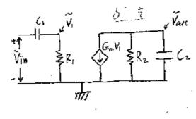
b) Plot amplitude and phase Bode plots when  $R_1$  = 10K $\Omega$ C<sub>1</sub>= 0.01  $\Xi$ ,  $R_2$  = 1K $\Omega$ C<sub>2</sub> = 0.001  $\Xi$ ,  $G_m$  = 0.01 S. (10 pts for each plot).
