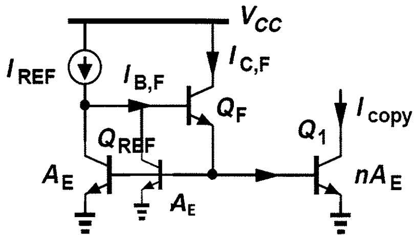
$$I_{\text{REF}} = I_{\text{BF}} + 2 I_{\text{C}_{\text{REF}}} \quad - \textcircled{1}$$
