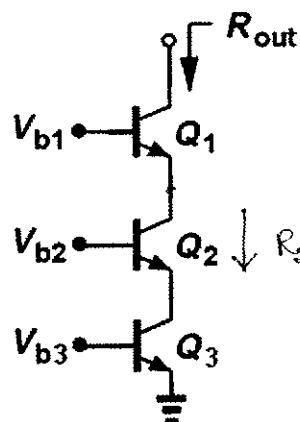
$$R_{out} = r_{o1} + (1 + g_m r_{o1}) \left\{ r_{\pi_1} || R_2 \right\} \approx g_m r_{o1} (r_{\pi_1} || R_2)$$
