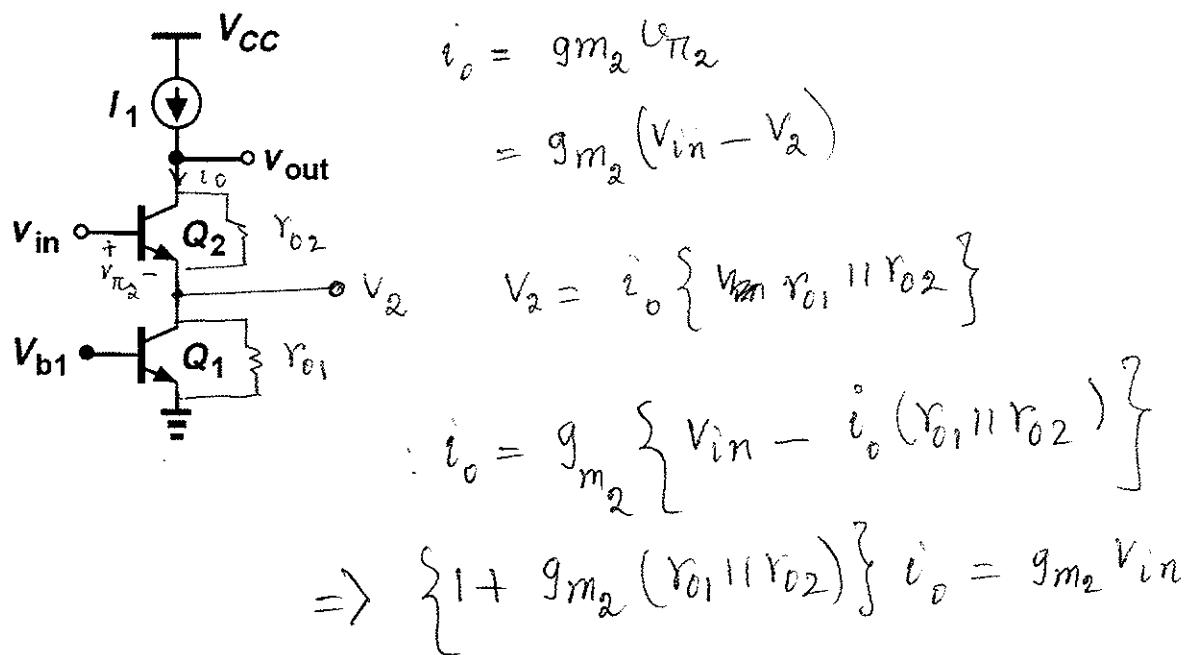
$$\therefore G_m = \text{overall gain} = \frac{i_o}{v_{in}}$$
