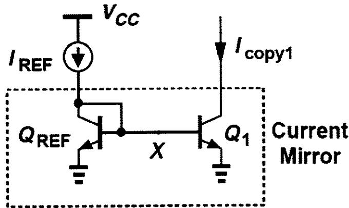
$$V_x = V_T \ln \left( \frac{I_{\text{copy}1}}{I_{S1}} \right) = V_T \ln \left( \frac{I_{\text{REF}}}{I_{S\text{REF}}} \right)$$
