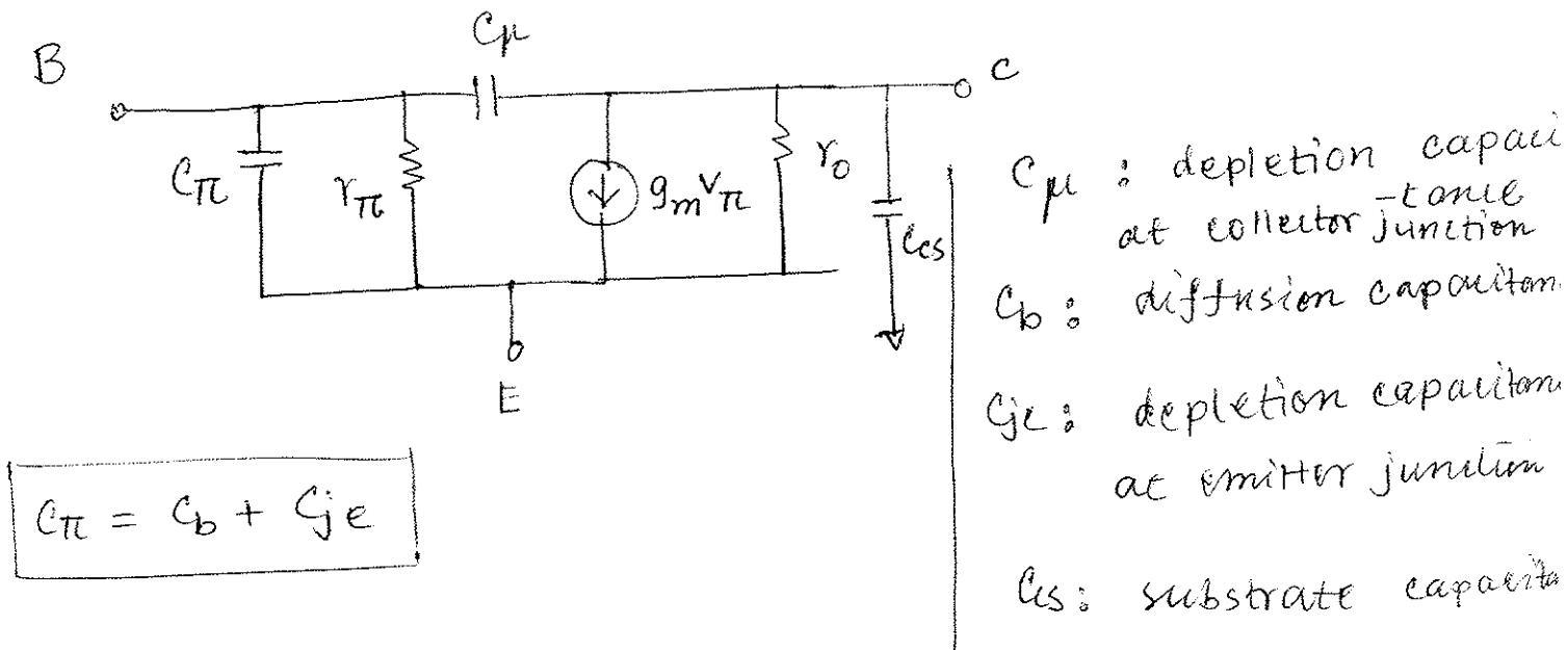
$C_{pe}$ : depletion capacitors at collector junction
