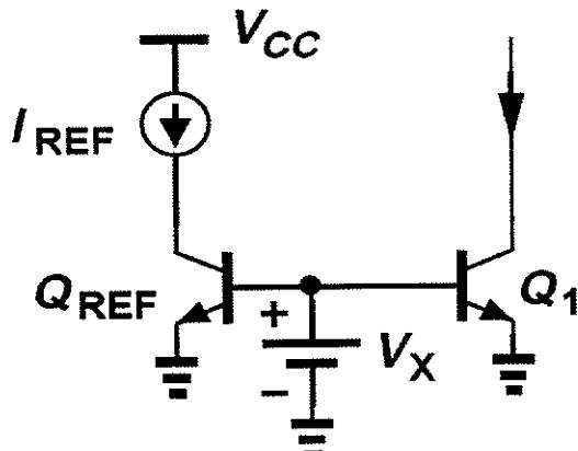
Since  $V_x$  is fixed,  $I_{\text{REF}}$  a change in temp will affect  $I_{\text{copy}1}$ . Note that without the diode connection  $\text{Q}_{\text{REF}}$  and  $\text{Q}_1$  are completely independent.  $V_c$  for  $\text{Q}_{\text{REF}}$  can be different than  $V_c$  at  $\text{Q}_1$ .
