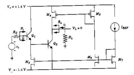
Given:  $I_{REF} = 100 \text{ (mu)A}$ ,  $V_L = 0 \text{(DC)}$ ,  $R_S = 1 \text{ k(omega)}$ ,  $R_L = 400 \text{ k(omega)}$ MOSEFTs:  $(W/L)_{3,5,6,7} = 10 \text{ and } (W/L)_4 = 25$
