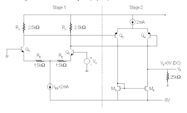
(a) [2 points] Draw the differential half circuit for Stage 1.
