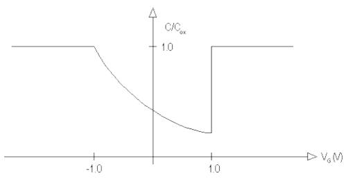
A MOS C-V curve is shown above for an n+ polysilicon gate and a p-type substrate, with Na=1E-16 cm&#175 &#179.
