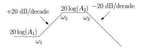
The frequencies are  $\omega_1 = 20\pi$ ,  $\omega_2 = 200\pi$ , and  $\omega_3 = 2000\pi$ . The gains  $A_1$  and  $A_2$  are positive. The following expressions are offered as potential transfer functions for the Bode plot:
