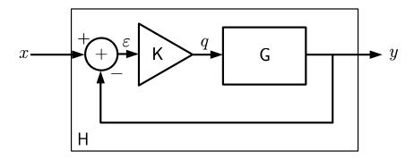
The input signal x represents a *desired* angular position. The output signal y is the *actual* angular position of the object; sensors determine the actual position and feed it back to be subtracted from the desired angular position x.
