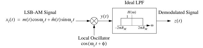
(Note that  $\hat{m}(t)$  denotes the Hilbert transform of m(t), and that the lowpass filter has a cutoff frequency equal to the bandwidth of m(t).) The local oscillator has a phase error  $\phi$ . Derive an expression for the demodulated signal z(t), and use it to explain whether the demodulator works well when  $\phi \neq 0$ . You can assume that m(t) is an audio signal and that  $\hat{m}(t)$  sounds very different from m(t). Hint: you may use the trigonometric identities:
