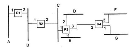
The network above uses CIDR addressing. A-G are subnets separated by the routers R1-R4.
