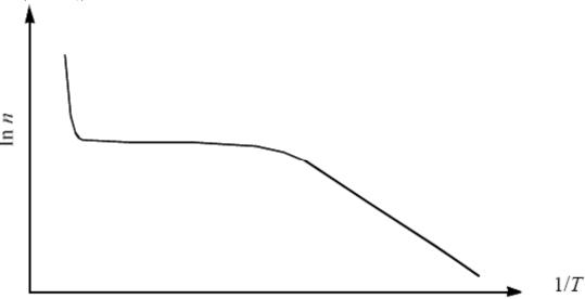
c) [5 pts] Draw a second curve that would correspond to another Si wafer, but doped with a different donor such that  $(E_D - E_C)_{NEW\_DONER} = 4 \text{ x } ((E_D - E_C)_{As}$ , where  $E_D$  is the donor energy level.
