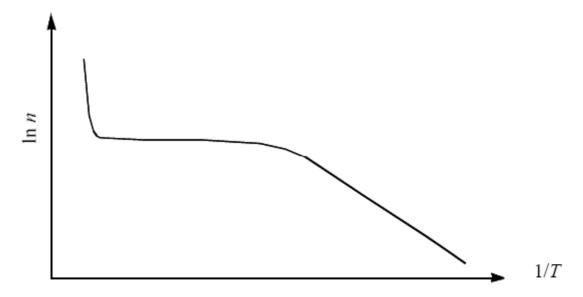
d) [ $5pts\ extra\ credit$ ] Draw a second curves that would correspond to a heavily doped Si wafer. Hint: when doping density is high, the impurity energy level splits into a band of available states due to Pauli exclusion principle. This impurity band crosses  $E_c$ .
