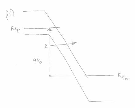
(iii) Tunneling. Electrons flow from p-side to n-side.
