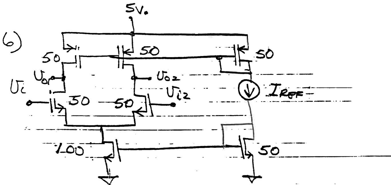
WHAT IS THE CURRENT,  $I_{REF}$ , WHICH GIVES A COMMON MODE REJECTION RATIO (CMRR) OF 60dB?
