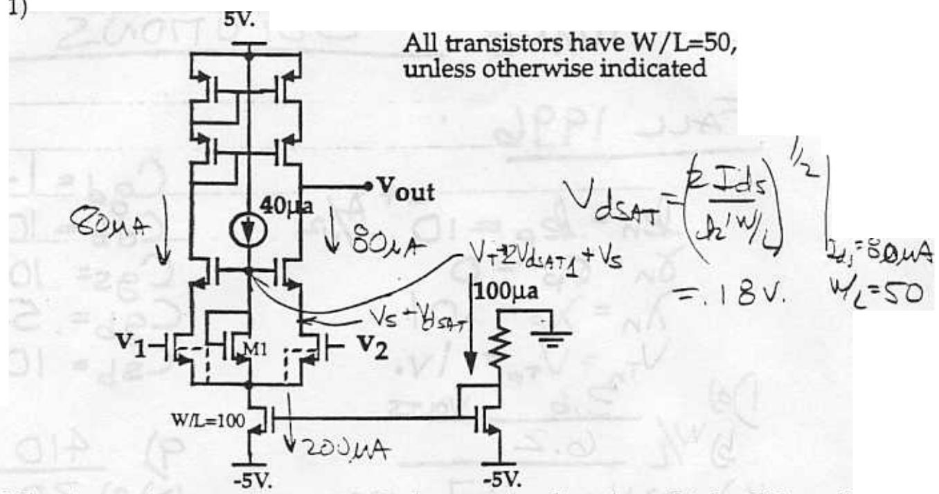
a) What is maximum value at  $v_{out}$  in the positive direction which still has all transistors in saturation?
