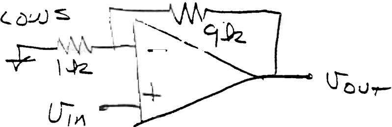
AT WHAT FREQUENCY SHOULD A COMPENSATION POLE BE ADDED SO THAT THE PHASE MARGIN IS  $45^\circ$ ? WE  $\frac{40}{\text{sec}} = 410 \text{ RAD/sec}$
