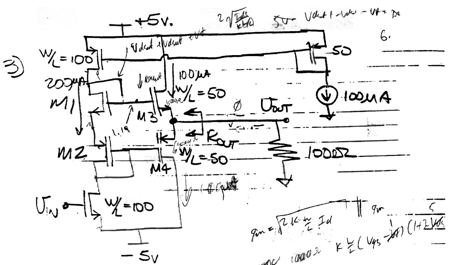
Q) Assume  $V_{in}$  is set so the output is at 0 Volts. What are the N/L's off  $M_1$  &  $M_2$  so that the output resistance,  $R_{out} = 500\Omega$ ?  $M_1 = 100$
