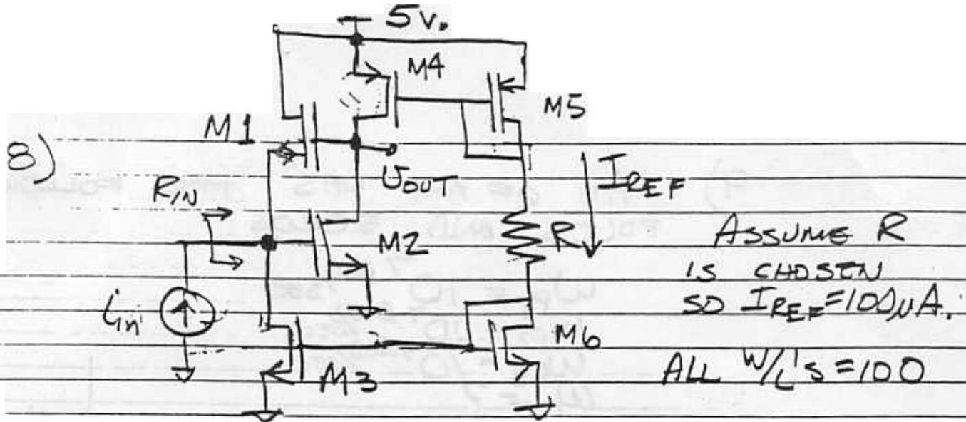
ANALYZE THIS CIRCUIT CONSIDERING M1 & M3 AS THE PROVIDING FEEDBACK AND M2 & M4 AS THE BASIC AMPLIFIER
