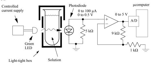
The 5 k $\Omega$  resistor in parallel with the photodiode converts 100  $\mu A$  into 0.5 V. A larger value will cause saturation at the forward voltage of about 0.6 V. A much smaller resistor will decrease the signal and reduce the signal-to-noise ratio. The noninverting amplifier provides a voltage gain of 10. A smaller resistor was okay, so long as the gain-resistance product was 50 k $\Omega$ .
