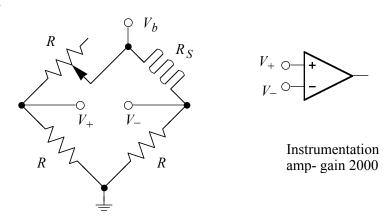
$$V_{+} - V_{-} = V_{b} \left( \frac{R}{2R} - \frac{R}{2R + \Delta R} \right) = V_{b} \left( \frac{\Delta R}{4R + 2\Delta R} \right) \approx V_{b} \left( \frac{\Delta R}{4R} \right) = V_{b} \left( \frac{G_{S}}{4} \right) \left( \frac{\Delta L}{L} \right) = V_{b} \left( \frac{\Delta L}{2L} \right)$$
