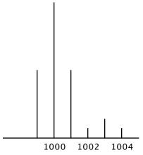
**1.11** A sinewave of frequency 4M - 84,000 Hz = 178,144 Hz will produce non-zero coefficients at  $H_{20999}$ ,  $H_{21000}$ ,  $H_{21001}$ ,  $H_{M-20999}$ ,  $H_{M-21000}$ , and  $H_{M-21001}$ .
