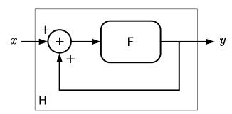
(i) Determine the frequency response  ${\cal H}(\omega)$  of the composite system.
