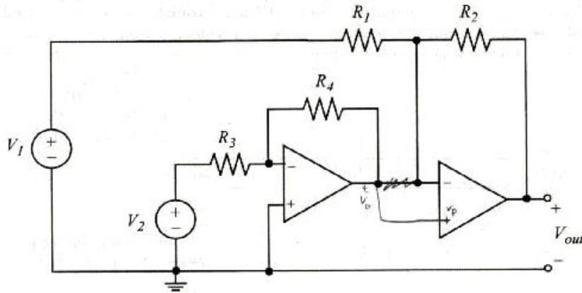
Find  $V_{out}$  in terms of  $V_1$ ,  $V_2$ ,  $R_1$ ,  $R_2$ ,  $R_3$ ,  $R_4$ . [10 pts]
