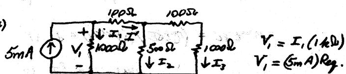
$$R_{eq} = \left\{ \left[ \frac{(100+1000)}{1100} \parallel 500 \right] + 100 \right\} \parallel \left( \frac{1000}{1000} \parallel 100 \right) = 144 \parallel 100 = 307\Omega \Rightarrow I_1 = \frac{V_1}{1k\Omega} = \frac{(5mA)(R_{eq})}{1k\Omega} = 1.54mA.$$
