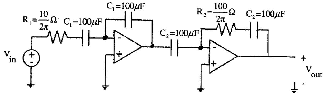
a. (15 pts) Let  $R_1 = 10/(2\pi)$  ohms,  $R_2 = 100/(2\pi)$  ohms,  $C_1 = 100 \mu F$ , and  $C_2 = 100 \mu F$ . Show that the transfer function of the circuit shown above is:
