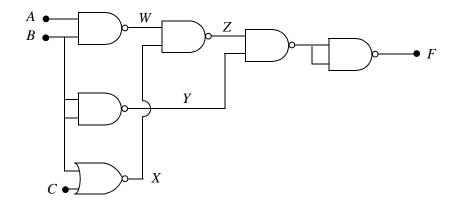
(a) Fill out the truth table (opposite), showing the intermediate values W, X, Y, Z as well as the output F.
