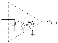
(b) For the circuit shown below, neatly and carefully sketch the voltage at node X and the output on the page opposite. The amplifier is a high-gain amplifier with a gain of greater than a million, an input resistance of greater than  $1M\Omega$ , and an output resistance of less than  $100\Omega$ .
