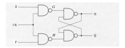
Fill in the value for Q in the timing diagram opposite. But to show your work, you must also show values for G and H. Note that the initial value of Q is 0, as shown by heavy dark line on the timing diagram. Ignore stage delay.
